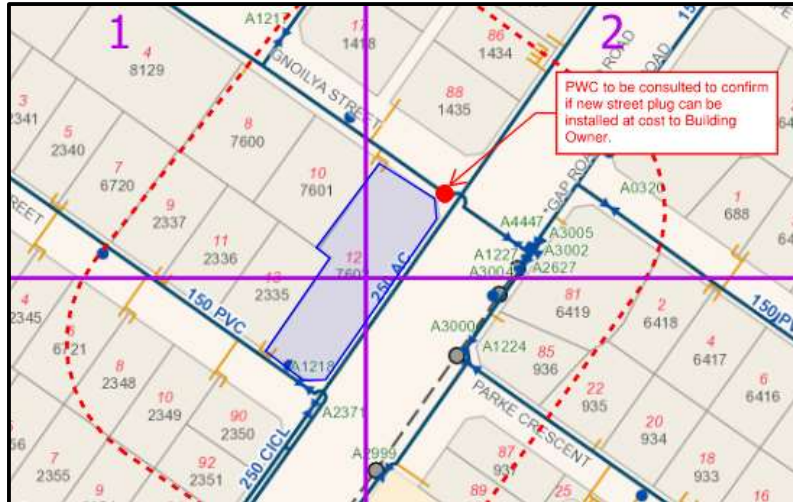
Figure 25 - Indicative Location of New Street Hydrant (Gnoilya Street main). Subject to PWC.
