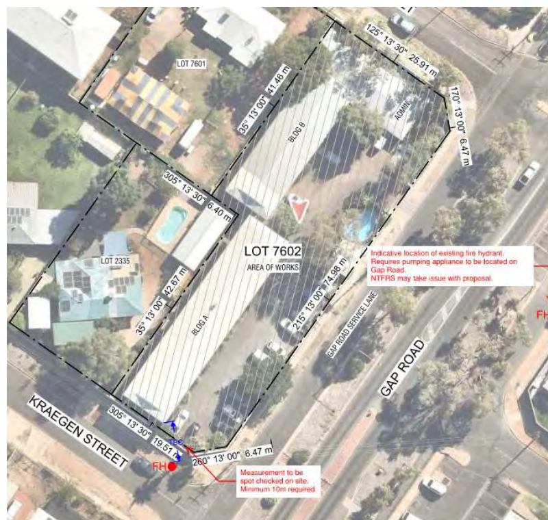
Figure 24 Existing Fire Hydrant Locations
