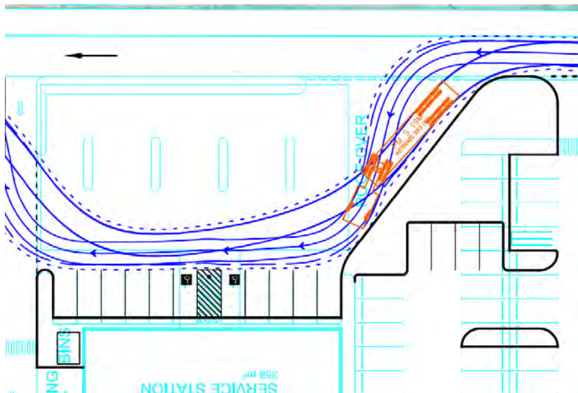
Figure 18 – example design of a loading space for the 19.0 m semi-articulated truck at the service station
